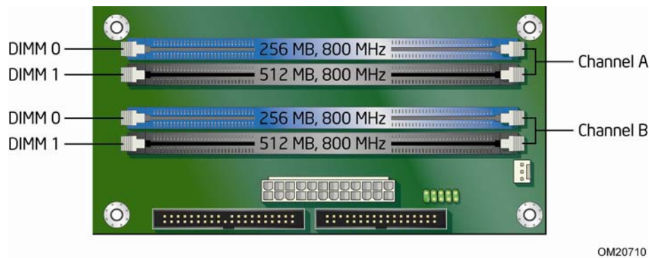
Figure 14. Dual Channel Memory Configuration with Four DIMMs
